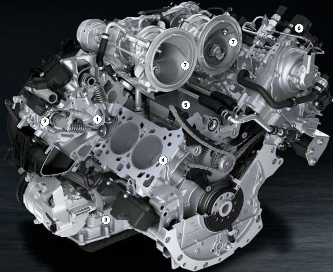
2.9-liter twin-turbo V6 engine in the Macan Turbo.
